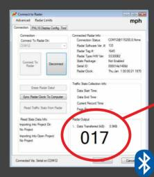
Constantly updating speed output transmitted to the remote computer via optional Bluetooth signal.
